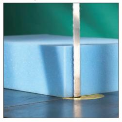
A V-shaped toothed bandknife available in single or double edge with teeth per inch (tpi) from 3 tpi to 20 tpi. Used to cut more rigid or higher density foam, the teeth give greater penetration to the cut. Toothed bandknives can also be used for cutting abrasive foam or any similar application where a straight edged blade would wear quickly. They also offer extended blade life where the machine is not fitted with a resharpening attachment. Available in widths from 10mm to 32mm.
