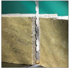
Notch edge and angle notch edge bandknife is used for some very specialised foam cutting applications and also for coating with grit or diamond. Available in widths from 10mm to 38mm.
