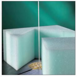
A range of narrow bandknives for cutting contours on fully automated CNC machines or on manual machines. Available in straight edge or toothed edge and in widths from 3mm to 4.5mm. Can be produced as continuous loops or as straight lengths for reciprocating machines.
