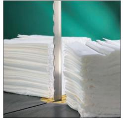
A wavy edge bandknife for cutting materials such as tissue, paper and textiles, the wavy edge gives a clean, smooth finish. Available in widths from 13mm to 25mm and in a short wave pitch or long wave pitch.
