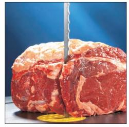
A scallop edge bandknife for many food slicing applications including boneless meats, processed meats, cheeses and soft-boned meats. Also used for cutting rubber seals and gaskets, packaging material and other applications where an initial penetration is needed. Available in widths from 10mm to 25mm with various pitches and gullet depths.
