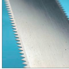
A specialist bandknife blade manufactured to fixed lengths. Available in widths from 10mm to 68mm and with tpi from 3 to 20. Used in the packaging industry and also for specialist foam manufacturing machinery.
